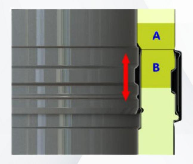
The flue gas temperature of a power geThe flue gas temperature of a power generator engine can reach 600°C. Since the material of the inner wall is stainless steel, it experiences a thermal expansion of approximately 10 mm per meter. In the Dinak GE+ system, thermal expansion is absorbed by each joint between elements, as indicated in the picture on the side.
